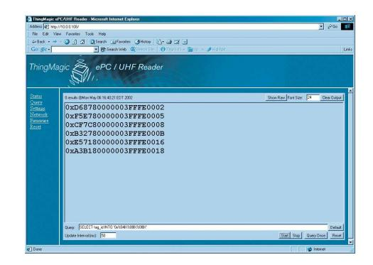
Figure 6: Java Reader interface – Query Page: Six aggregated EPC numbers are displayed in the browser window.
