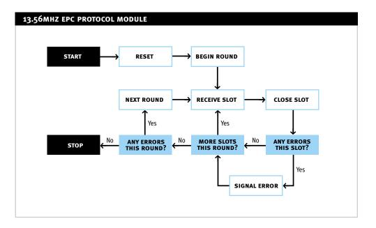
In addition, an error signal is sent if the Reader believes that the previous slot contained a tag response but was unable to decode it properly. This error signal informs the tag that its response was not successfully received and that it should repeat its response later (during the next round.)
